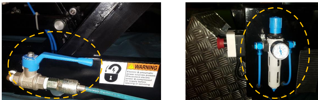
Figure 3-8 Pneumatic Connection at Mainframe machine assembly
