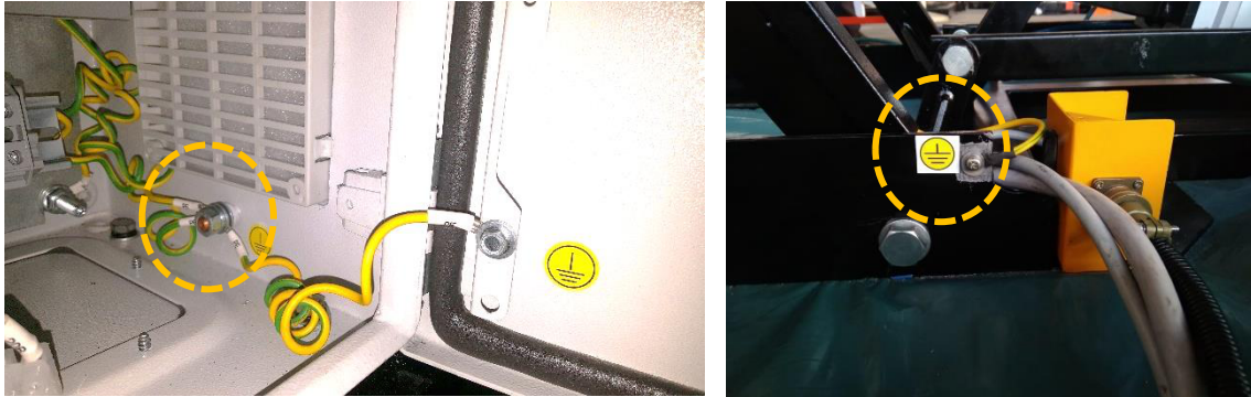
Figure 3-7 PE / Ground connection on Panel and Machine
