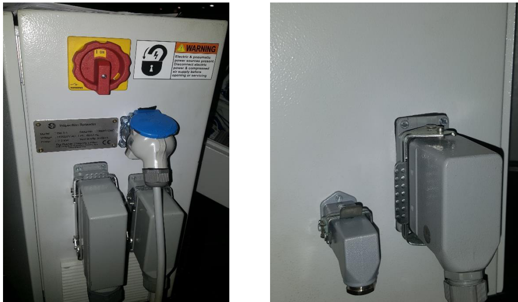
Figure 4-1 Connectors in Panels
