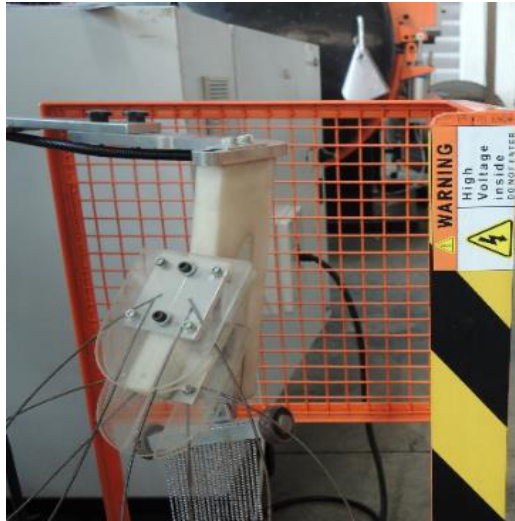
Figure 4-10 Guard to avoid impact hazard
