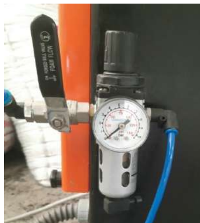
Figure3-7 Pneumatic Connection at Main frame machine assembly
