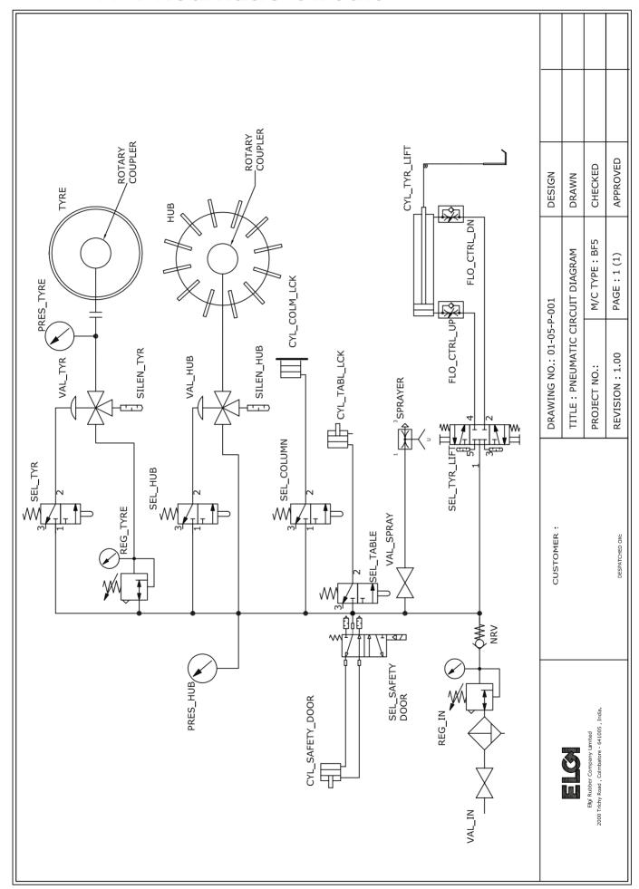
22 \_\_\_\_\_\_\_ 11 Pneumatic Circuit
